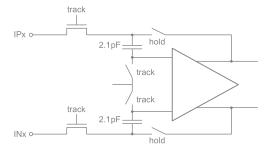
Figure 2. Input Configuration
