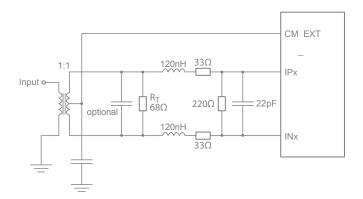
Figure 6. Alternative Input Network
