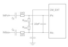
Figure 5. AC-Coupled Input
