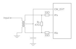
Figure 4. Transformer-Coupled Input
